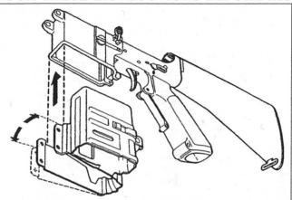
Slide the REDI-MAG clamp around the magazine housing of the rifle. Bend the right arm of the clamp slightly outward until it clears the raised lip around the bottom of the magazine housing. Be careful not to scratch the aluminum finish on the rifle, as the steel used in the REDI-MAG is very hard and tough. NOTE: While it is possible to install the REDI-MAG without disassembling the lower receiver assembly from the upper receiver assembly, it is easier to install if the receiver assemblies
