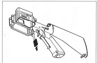
Slide the Rear Gasket (small rectangular) between the front arch of the trigger cut-out and the rearmost, curved portion of the REDI-MAG clamp.
