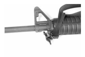
It looks like this when done. It is now silent and secure, and the wire inside the loop prevents melt through.
